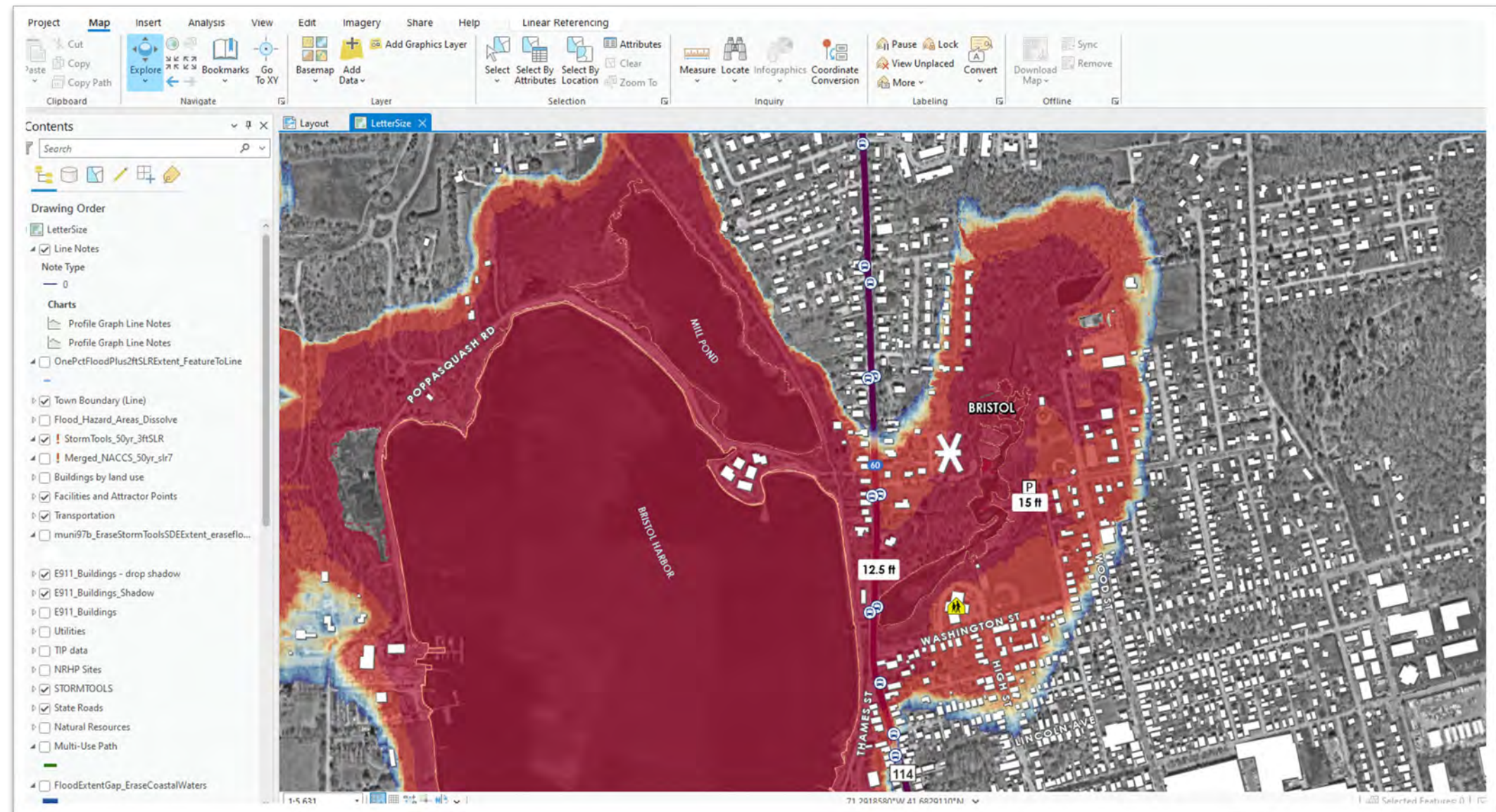
Example ArcGIS screenshot showing depth of flooding along Route 114 in Bristol
